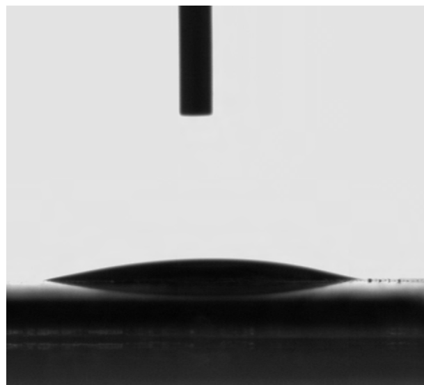
Fig. 5. Photograph of water droplet shape on a ZnO nanoflower film.
